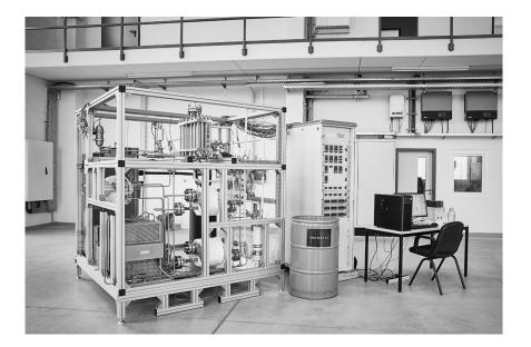
INERATEC used six Vahterus heat exchangers in their Power-to-Liquid Hot Box. In the INERATEC Gas-to-Liquid, Power-to-Liquid and Power-to-Gas processes, the compact and intelligent design of heat exchangers is essential for high thermal efficiency. Heat recovery and compact heating, as well as cooling at different points within the synthesis process are key design features in the container-sized plants.
