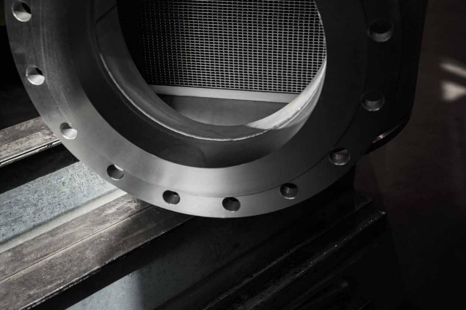
Shell side view of new 5SH plate pack. Instead of the round shape of the original plate, the new plates use the shape of an athletics field.
