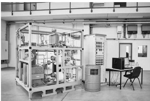
INERATEC used six Vahterus heat exchangers in their Power-to-Liquid Hot Box.
