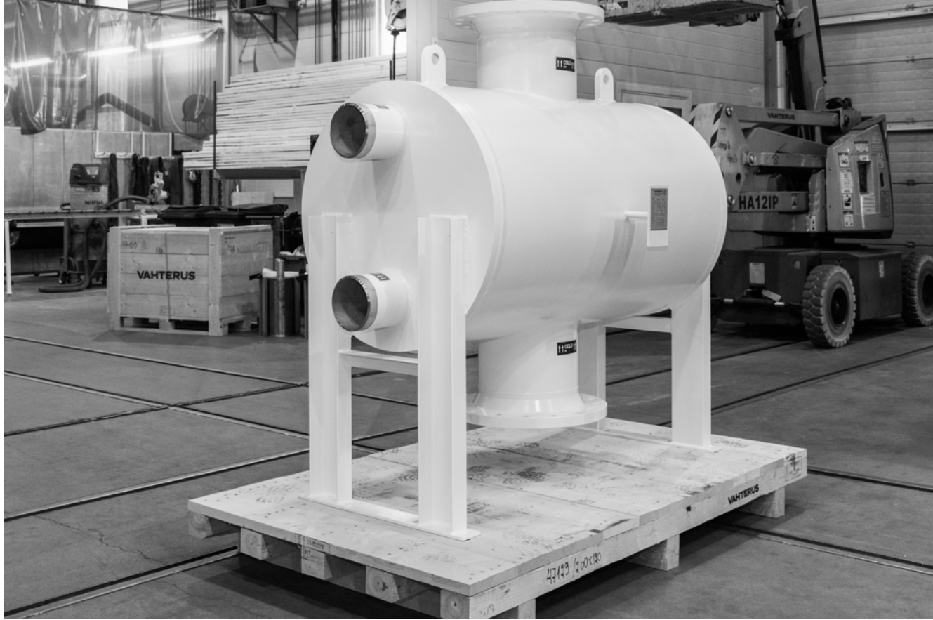
Pölkky replaced an old tube heat exchanger in Taivalkoski production unit with a fully welded 12-MW Vahterus Plate & Shell heat exchanger. The compact size makes it easier to install in a production plant.
